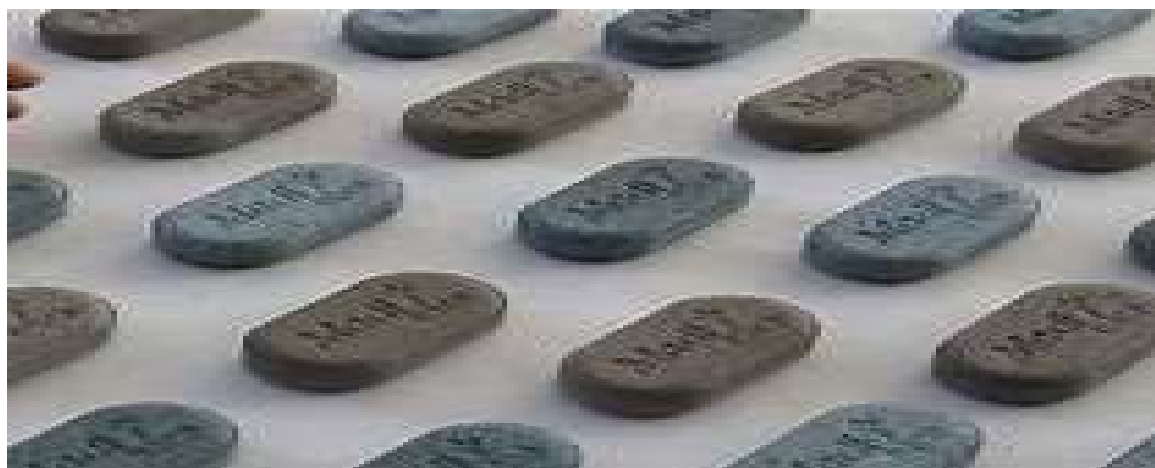
Figure 18: The picture of Madi Drop+ that was placed in the bucket for water treatment.
