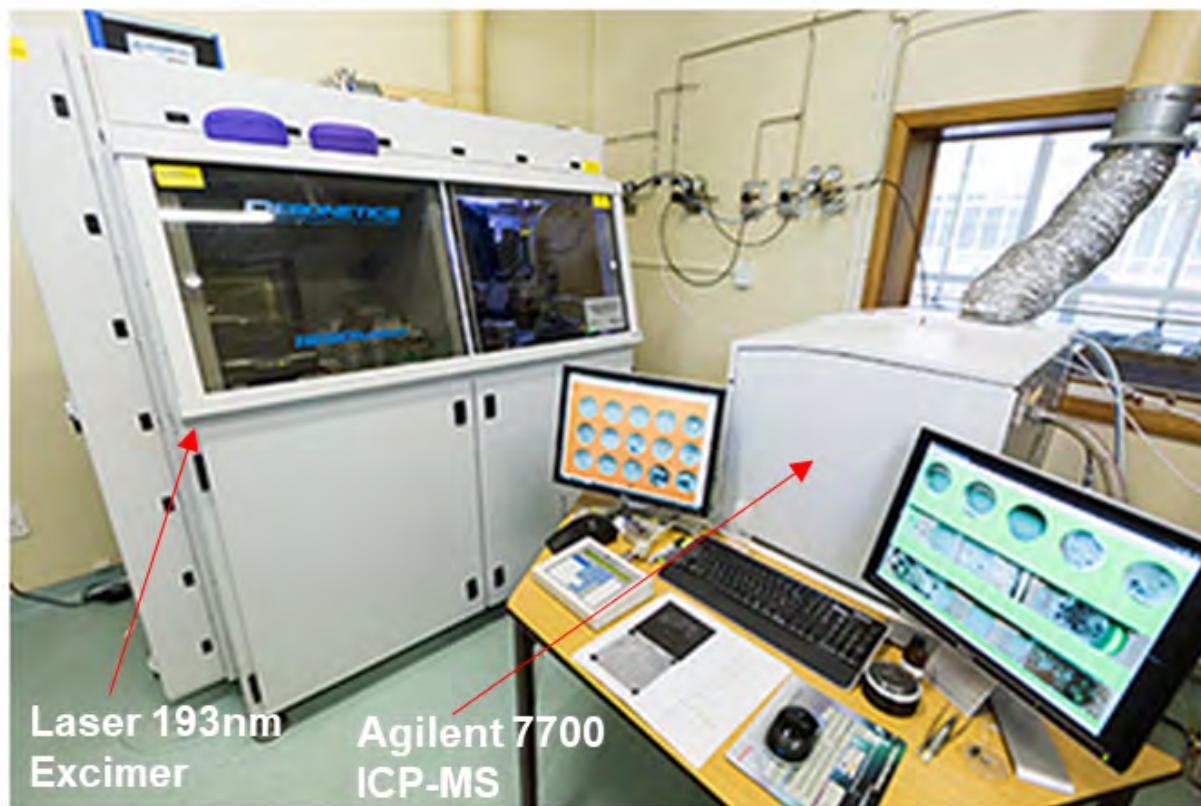
Figure 3.6: Laser 193 nm Excimer interfaced to the Agilent 7700 ICP-MS.
