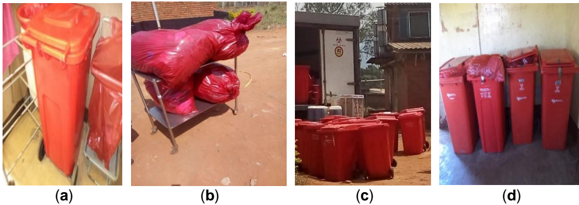
Figure 4.5. Onsite transportation of HCRW: Wheelie bin in the sluice room of a healthcare facility (a); medication trolley being used to transport HCRW to the central storage area (b); HCRW being transported out of healthcare facility with wheelie bins (c) and overfull wheelie bins and some with faulty locks (d). (Source: Field work).
