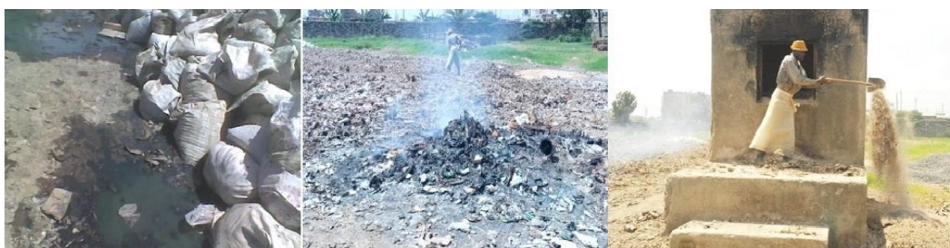
Figure 3: Tannery wastes crudely dumped in sacks and burnt in the open space and kiln in a tannery in Kenya (Oruko, 2017).
