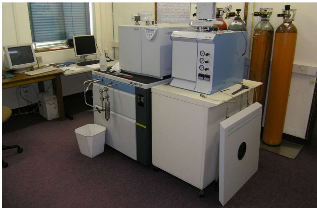
Figure 3.15: Finnigan Delta XP Mass Spectrometer with a dual gas inlet.
