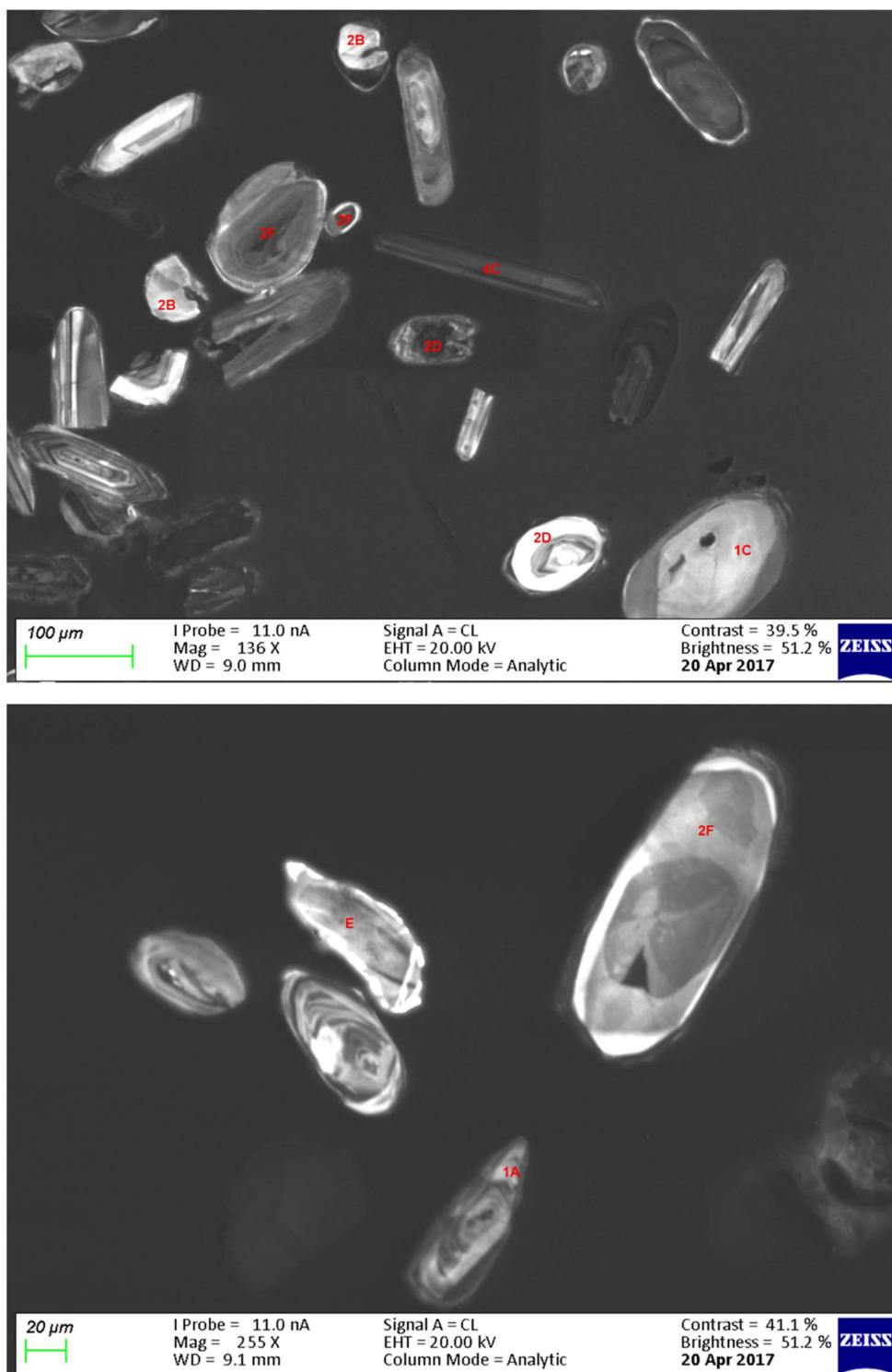
Figure 7.1b: CL images of some of the representative zircons showing main types of internal structures within the studied Lakiri kaolins where, 1: Euhedral; 2: Subhedral to subrounded grains; 4: Needle-like grains; A: Oscillatory/growth zoning; B: Sector zoning; C: Homogeneous unzoned; D: Chaotic texture; E: Irregular concentric zoning; and F: Xenocrystic cores.
