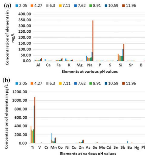
Fig. 14. Concentration of elements in treated water at various equilibrium pH: (a) in mg/L and (b) in  $\mu\text{g/L}$ . Initial  $F^-$  concentration = 8 mg/L, volume of solution = 50 mL, adsorbent dosage = 0.4 g, initial pH 2, temperature = 298 K and shaking speed = 200 rpm.
