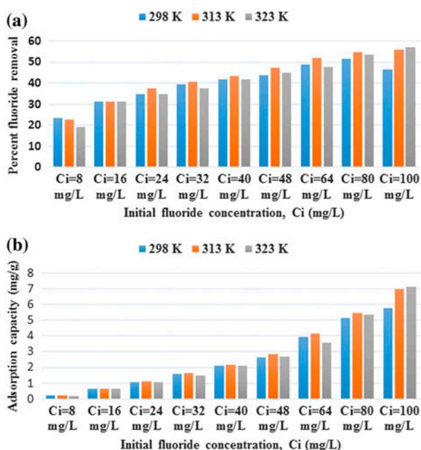
Fig. 9. Variation of (a) per cent fluoride removal and (b) adsorption capacity with temperature. Volume of  $F^-$  solution = 50 mL, contact time = 30 min, initial pH 2, adsorbent dosage = 0.4 g and shaking speed = 200 rpm.
