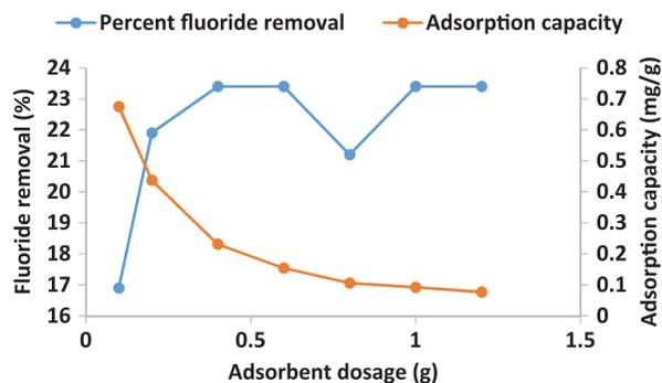
Fig. 6. Variation of a per cent fluoride removal and adsorption capacity with adsorbent dosage. Initial F<sup>-</sup> concentration = 8 mg/L, volume of solution = 50 mL, contact time = 30 min, temperature = 298 K, initial pH 2 and shaking speed = 200 rpm.
