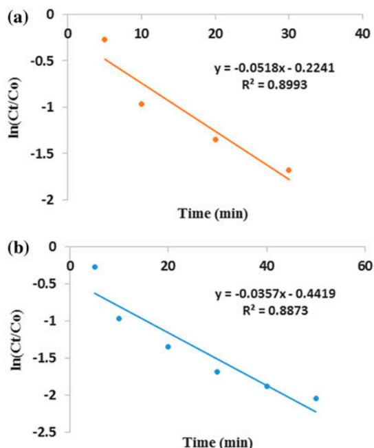
Fig. 12. External diffusion plots (a) for contact time up to 30 min and (b) for all contact time. Initial  $F^-$  concentration = 8 mg/L, volume of solution = 50 mL, adsorbent dosage = 0.4 g, initial pH 2, temperature = 298 K and shaking speed = 200 rpm.
