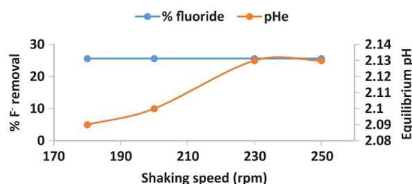
Fig. 4. Per cent fluoride removal as a function of shaking speed. Initial F<sup>-</sup> concentration = 8 mg/L, volume of solution = 50 mL, adsorbent mass = 0.4 g, contact time = 30 min and temperature = 298 K.
