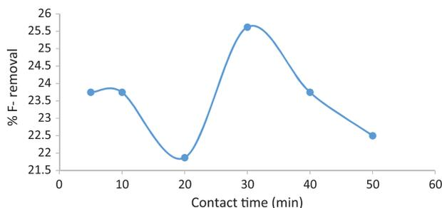
Fig. 5. Variation of per cent fluoride removal with contact time. Initial F<sup>-</sup> concentration = 8 mg/L, volume of solution = 50 mL, adsorbent dosage = 0.4 g, temperature = 298 K, initial pH 2 and shaking speed = 200 rpm.
