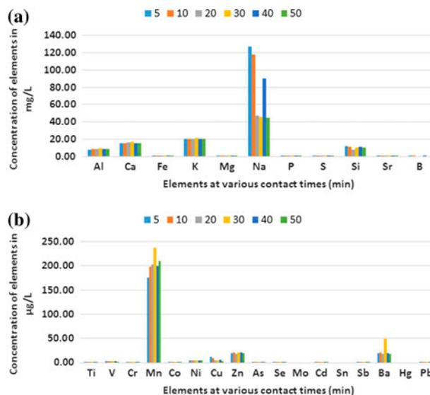
Fig. 13. Concentration of metal and non-metal species in treated water at various contact times: (a) in mg/L and (b) in  $\mu\text{g/L}$ . Initial  $F^-$  concentration = 8 mg/L, volume of solution = 50 mL, adsorbent dosage = 0.4 g, initial pH 2, temperature = 298 K and shaking speed = 200 rpm.
