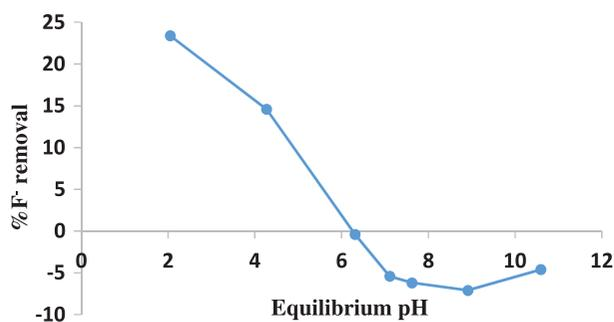
Fig. 7. Variation of per cent fluoride removal with equilibrium pH. Initial F<sup>-</sup> concentration = 8 mg/L, volume of solution = 50 mL, contact time = 30 min, temperature = 298 K and shaking speed = 200 rpm.
