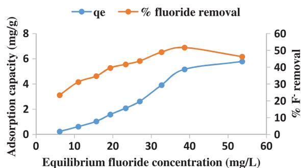
Fig. 8. Variation of adsorption capacity and per cent fluoride removal with equilibrium fluoride concentration. Volume of F<sup>-</sup> solution = 50 mL, contact time = 30 min, initial pH 2, adsorbent dosage = 0.4 g and shaking speed = 200 rpm.
