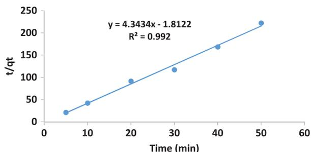
Fig. 11. Pseudo-second-order plots for defluoridation at different contact times. Initial  $F^-$  concentration = 8 mg/L, volume of solution = 50 mL, adsorbent dosage = 0.4 g, initial pH 2, temperature = 298 K and shaking speed = 200 rpm.
